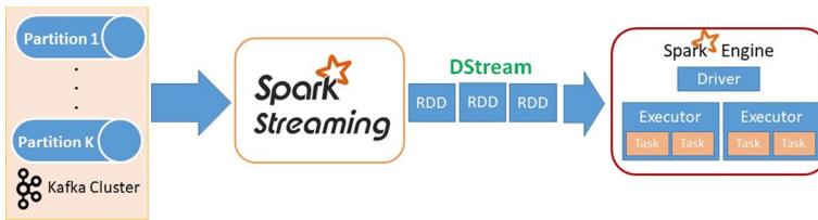
Fig. 3 Workflow of video processing with Kafka and Spark Streaming
