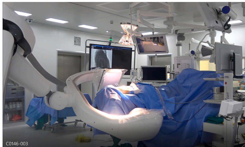
Fig. 7. The robot used to perform the 3D CT scan.
